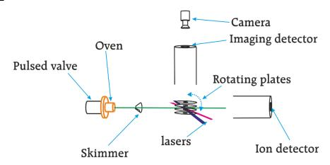
The "FEMTO" experiment is designed to monitor the time-resolved relaxation dynamics of molecular systems by mean of the photoelectron/ion spectroscopy or the mass spectroscopy. It couples a pulsed valve and a Velocity Map Imaging Spectrometer with two femtosecond laser pulses delayed as for a pump/probe scheme.
